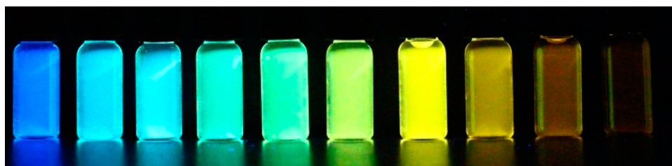
Figure 4. Emission solvatochromism of compound 5d (recorded in cyclohexane, toluene, THF, EtOAc, acetone, \text{CH}_2\text{Cl}_2 , MeCN, i PrOH, EtOH, MeOH (from left to right); T = 293\text{ K} ; c(\mathbf{5d}) = 10^{-4}\text{ M} ; \lambda_{\text{excit}} = 356\text{ nm} , hand-held UV lamp).
